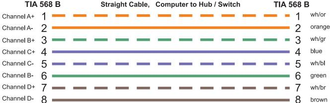
These cable and pin layouts are working equally well in all Ethernet environments as 10 Base-T, 100 Base-T and 1000 Base-T.
