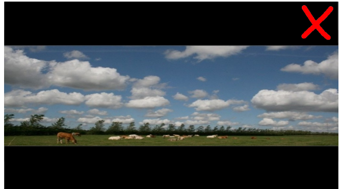
Figure 8 1:2.35 material letterboxed to a 4:3 SD tape format viewed on an uncompensated 16:9 screen
