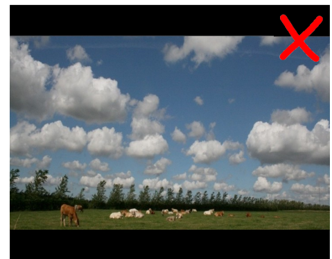
Figure 11 1:2.35 material formatted in a 16:9 widescreen letterboxed SD tape format, viewed on an uncompensated 4:3 screen
