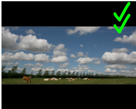
Figure 7 1:2.35 material letterboxed to a 4:3 SD tape format viewed on a 4:3 screen
