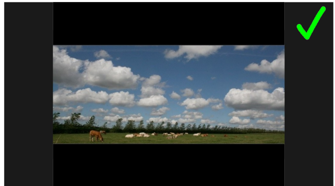
Figure 9 1:2.35 material letterboxed to a 4:3 SD tape format viewed on a 16:9 screen set to 4:3 mode
