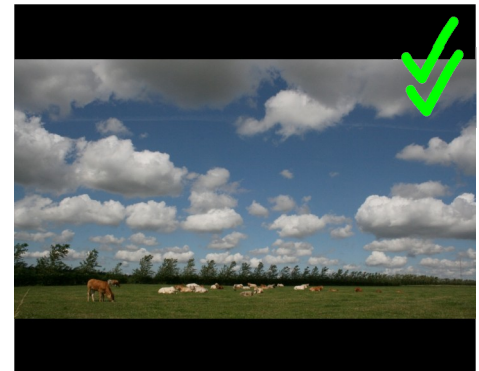
Figure 2 16:9 letterboxed picture from 4:3 SD tape format on 16:9 screen set to display 4:3
