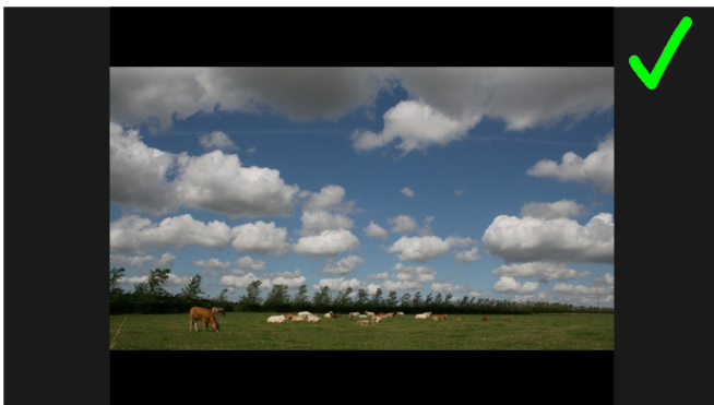
Figure 3 16:9 letterboxed picture from 4:3 SD tape format on 16:9 screen set to display 4:3
